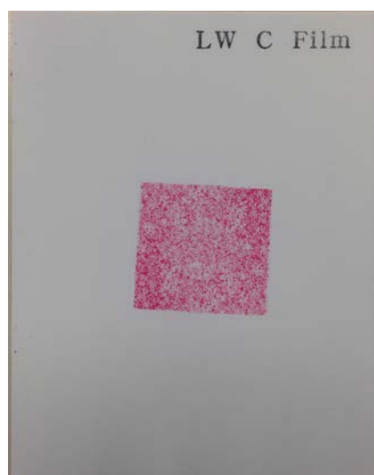
Fig. 13. The contour of the pressure measurement film after pressing.
