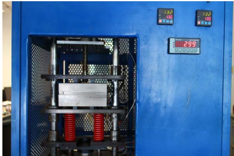
Fig. 11. The hot press machine during the desired operation.
