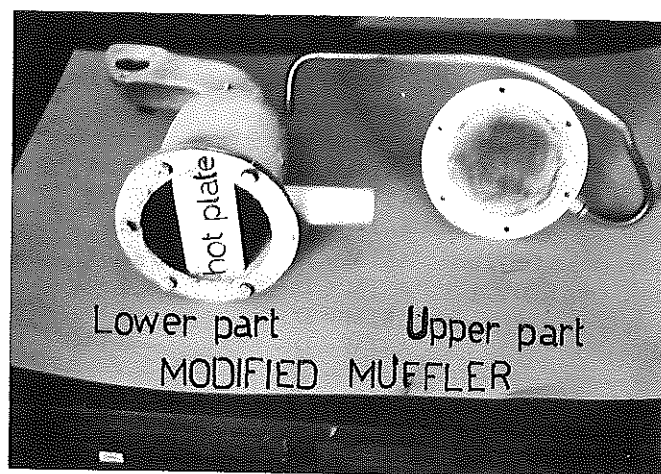
Fig. 2 Modified muffler has two parts, the upper acting as oil container and the lower as heater.
