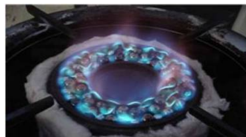
Fig. 6. Combustion in the porous medium of metal balls.
