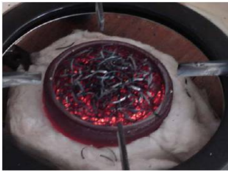
Fig. 7. Combustion in porous medium of metal chips.
