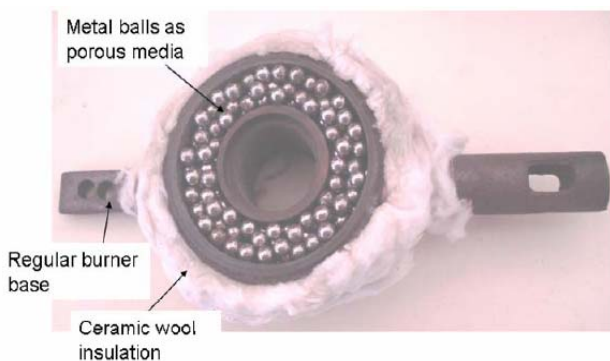
Fig. 5. Insulated mixing tube of a conventional burner filled with metal balls as porous media.
