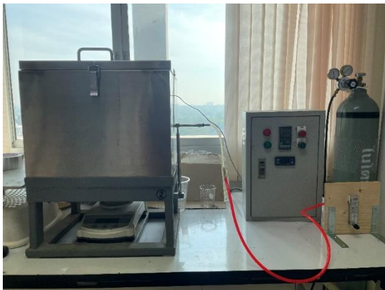
Fig. 2. Experimental setup (a) Torrefaction system (b) Reactor.
