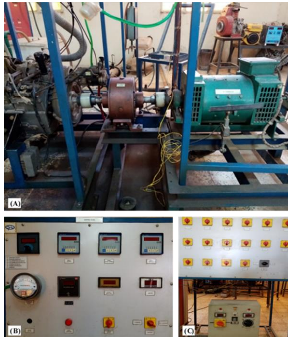
Fig 1. Setup of the test rig: (A) engine coupled with a motor, (B) load and speed measuring board, and (C) loading heaters and voltage and current measuring board.
